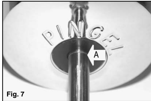
A: Center groove on cylinder shaft located at bottom of cylinder housing.
